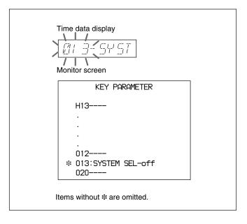
**2** Holding down the JOG/SHUTTLE button, turn the JOG/SHUTTLE dial to change the setting from "OFF" to "ON," then release the JOG/SHUTTLE button.
